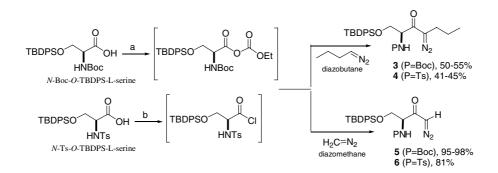
a: CICOOEt, Et<sub>3</sub>N, THF, -21-0°C, 30 min. Then, diazoalkane, 0°C-rt, 2h. b: CICOCOCl, CH<sub>2</sub>Cl<sub>2</sub>, 0°C-rt, 2h. Then, THF, diazoalkane, 0°C, 2h.
