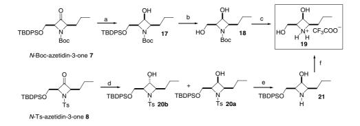
a: NaBH<sub>4</sub>, MeOH, -21°C, 30 min (46%). b: TBAF, THF, 0°C-rt, 3h (71%). c: TFA, CH<sub>2</sub>Cl<sub>2</sub>, 0°C, 1h (quantitative). d: NaBH<sub>4</sub>, MeOH, -21°C, 30 min (50% *cis* and 20% *trans*). e: Na/naphthalene/DME. f: TBAF, THF, 0°C-rt, 3h then, TFA (50%).
