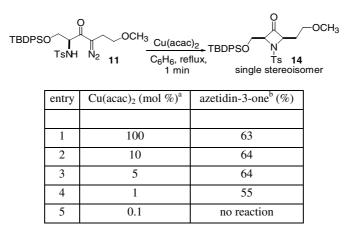
a.The catalyst was added as a solution in 0.65 mL of  $CH_2Cl_2$ . All the reactions were performed with 0.06 mmol of the diazo compound in 1.2 mL of  $C_6H_6$ ; b. Isolated yield.
